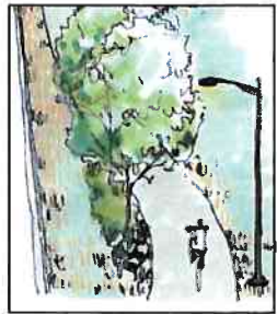
Potential curvilinear alignment creates wider "pockets" for landscape features in 140' right of way
